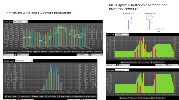
Figure 7 - Hybrid Power Plant EMS, wind, and PV power production forecast and MPO based batteries charge/discharge and inventory optimal schedule
