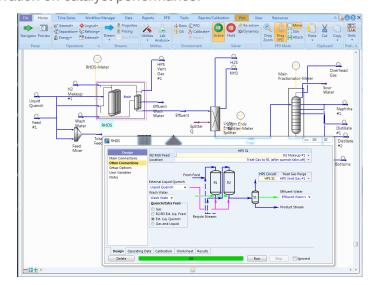
RHDS-SIM is a valuable tool to determine run lengths with different feeds, monitor deactivation, develop a consistent set of LP yield vectors and establish more profitable operations.
