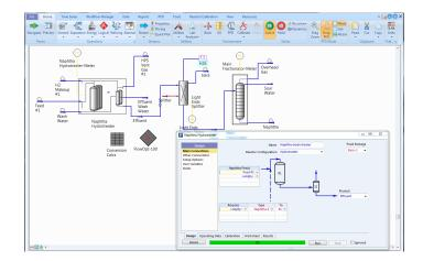
N HTR-SIM is a valuable tool to determine run lengths with different feeds, monitor deactivation, develop a consistent set of LP yield vectors and establish more profitable operations.
