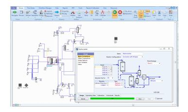
HCR-SIM is a valuable tool to determine the most profitable feeds and time to shutdown, to establish the best operating strategy, to monitor catalyst deactivation, and to develop a consistent set of yields vectors.
