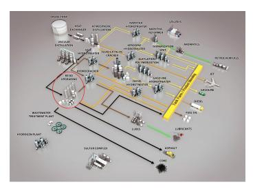
VIS-SIM, proven over decades of use with refineries worldwide, predicts yield and product properties based on the feed quality, furnace outlet temperature or severity, and unit geometry. The model predicts the key properties of the visbroken tar such as viscosity and stability. Detailed fractionation can be added upstream or downstream of the unit.
