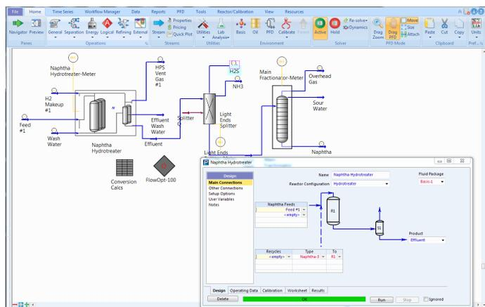
N HTR-SIM is a valuable tool to determine run lengths with different feeds, monitor deactivation, develop a consistent set of LP yield vectors and establish more profitable operations.
