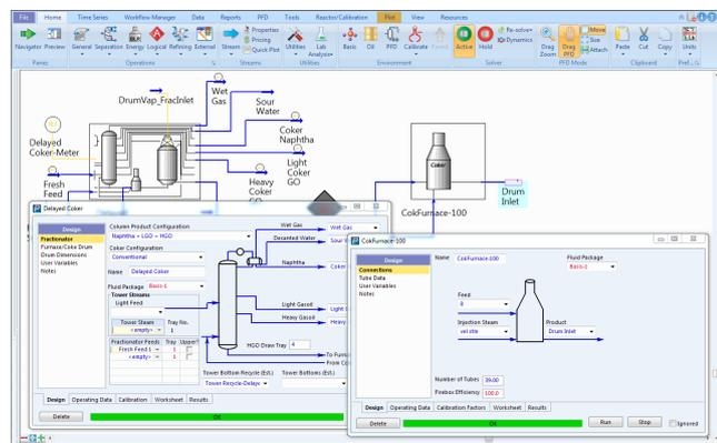
DC-SIM is a valuable tool to evaluate different crudes and their resulting coking yields on this key refinery process unit.
