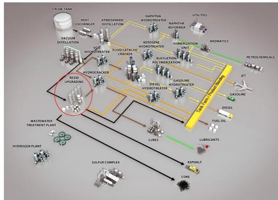
DC-SIM, proven through decades of use by refiners worldwide, allows you to model the impacts of a variety of different feedstocks such as atmospheric residuals, vacuum residuals, or FCC slurry. The simulation includes the furnace, drums, main fractionator, and the drum vapour quenching system. Cycle time (drum fill time) and resulting coke qualities are predicted.
